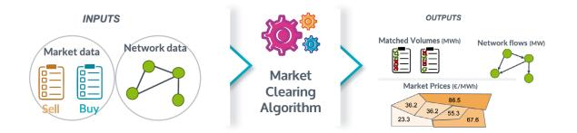
On the network data, it is often needed to find a trade-off between the accuracy of the grid representation and the complexity it adds to the power-matching algorithm.
